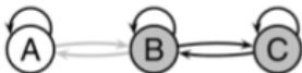
Fig. An HMM with two critical edges, A \rightarrow B and B \rightarrow A .
